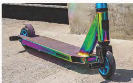
Alloy deck and steel brake, and 100 mm high impact wheels and durable ABEC-7 bearings.
